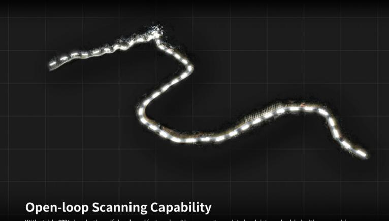
With stable RTK signals, the self-developed fusion algorithm generates point cloud data embedded with geographic coordinates, eliminating the need for closed-loop scanning. This enables the consistent delivery of point cloud data with absolute precision less than 5 cm.
