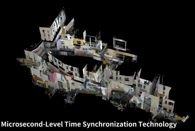
Empowered by SHARE's imaging algorithms, point cloud-image fusion algorithms, and multi-sensor microsecond-level time synchronization technology, the system achieves superior color accuracy and more authentic color reproduction in point clouds, ensuring relative accuracy up to 1 cm.
