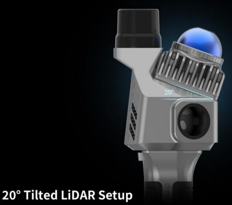
The LiDAR is angeled with a 20° tilt towards the ground, enabling comprehensive coverage of the ground, forward areas, and ceiling without manual repositioning. This setup boosts scanning efficiency, capturing all relevant areas in a single pass.
